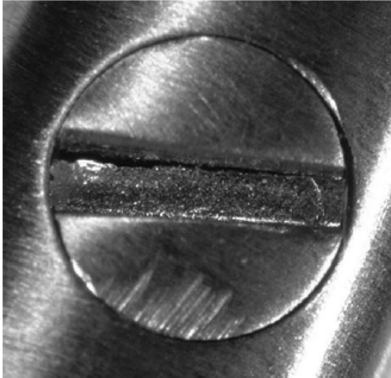
Figure 2 Magnified views showing a crack through the screw-head of fine scissors on the left, a cracked needle holder tip in the middle, and absence of solder to secure the jaw surface insert of a wire holder on the right.
