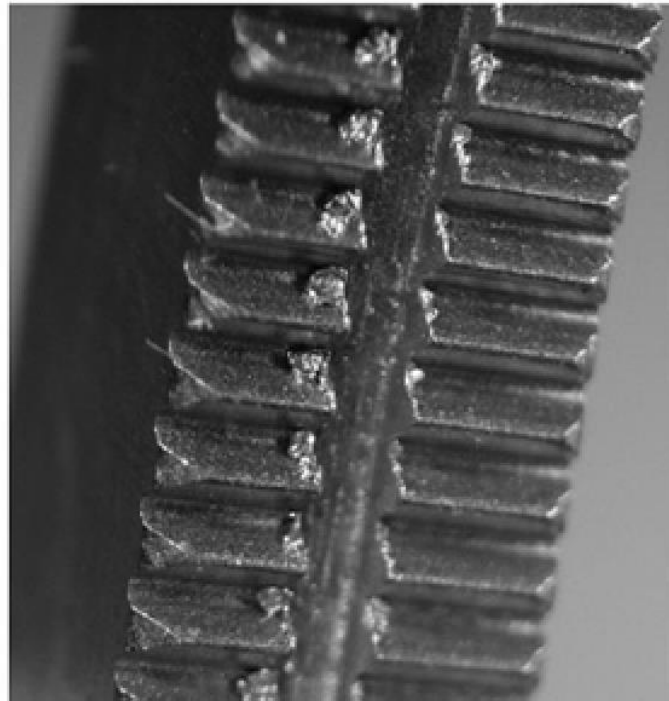
Figure 1 Magnified views of the jaws of vascular clamps – a well-finished example on the left, poorly finished examples in the middle and right views.
